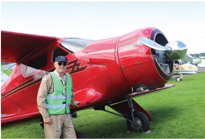
This flaming red beauty is a Beechcraft model 17, nicknamed Staggerwing. This name comes from the rare position of the wings. Unlike with most biplanes, the upper wing is positioned behind the lower one, what is called a 'negative wing stagger'.
